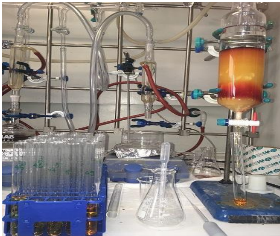
Figure 3. Column Chromatography using Selica gel and DCM solvent.
