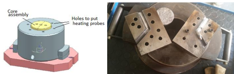
Figure 6. ECAP Die geometry and 120° intersected channels.
