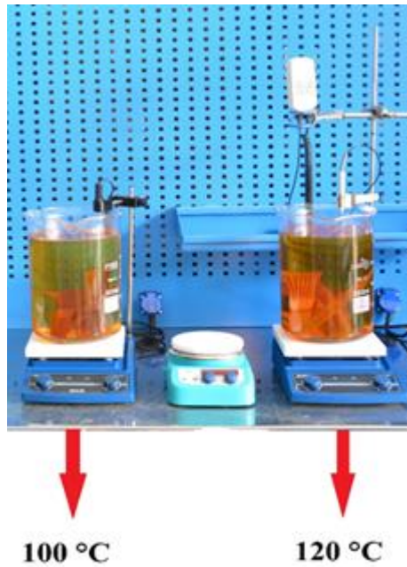
Figure 3. Specimens subjected to thermal ageing at different temperatures.
