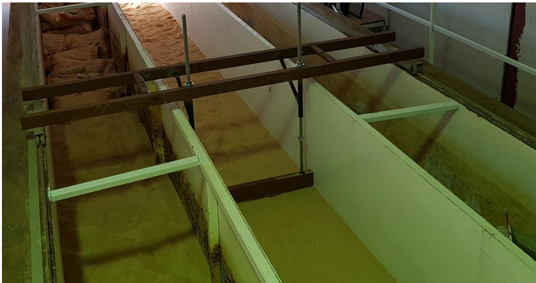
Figure 3.7 Apparatus to level the channel bed along the channel.
