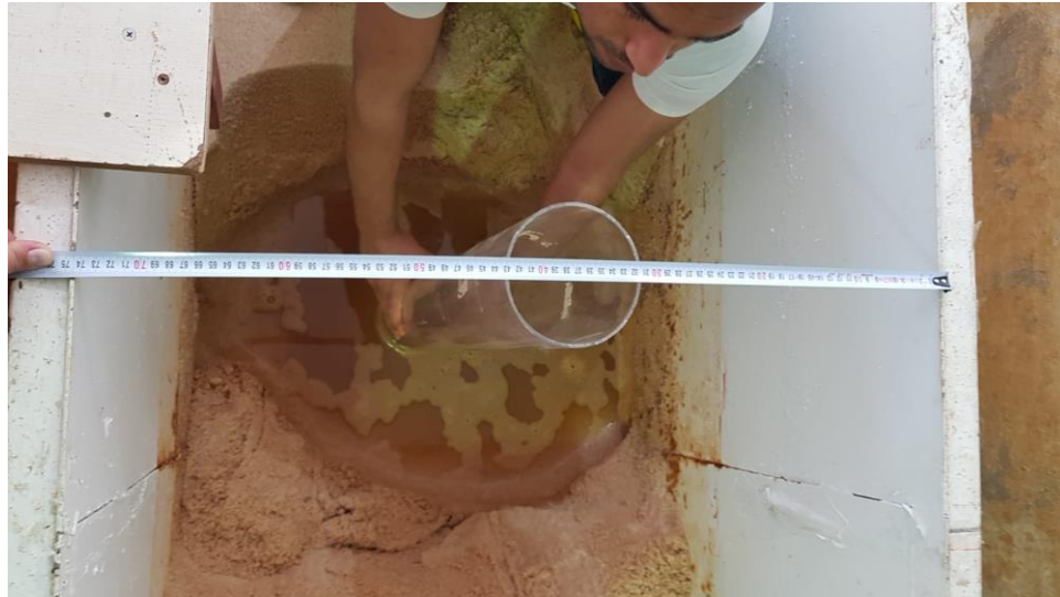
Figure 3.16 Pier is placed at the center of the channel.
