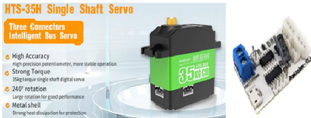
Figure 2.1: HTS-35H bus servo and its driver [19]
