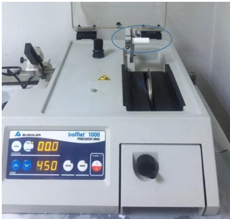
Figure 5: 1.65 mm thick slices (discs) were obtained by cutting under water-cooling with diamond blades (ISOMET 1000, Buehler).
