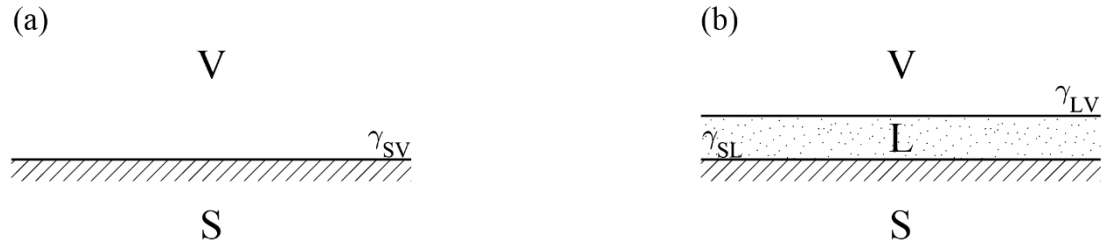
Figure 1.1: (a) Unwetted case: surface energy of solid vapor ( \gamma_{SV} ), (b) Wetted case: surface energies of liquid-vapor ( \gamma_{LV} ) and solid-liquid ( \gamma_{SL} )
