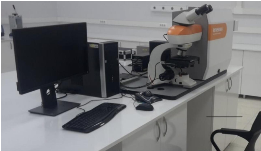
Figure 2.10: Raman spectroscopy device used in this study
