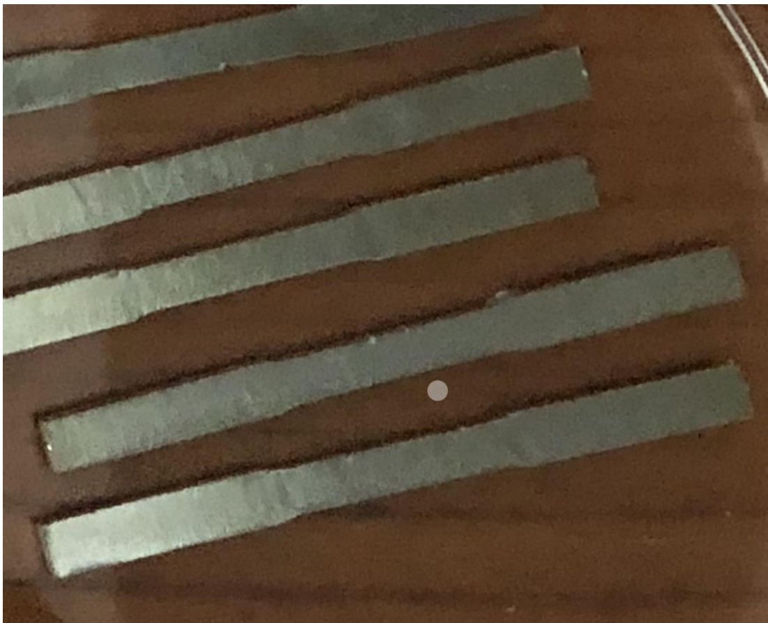
Figure 2.9: Tin coated aluminum samples
