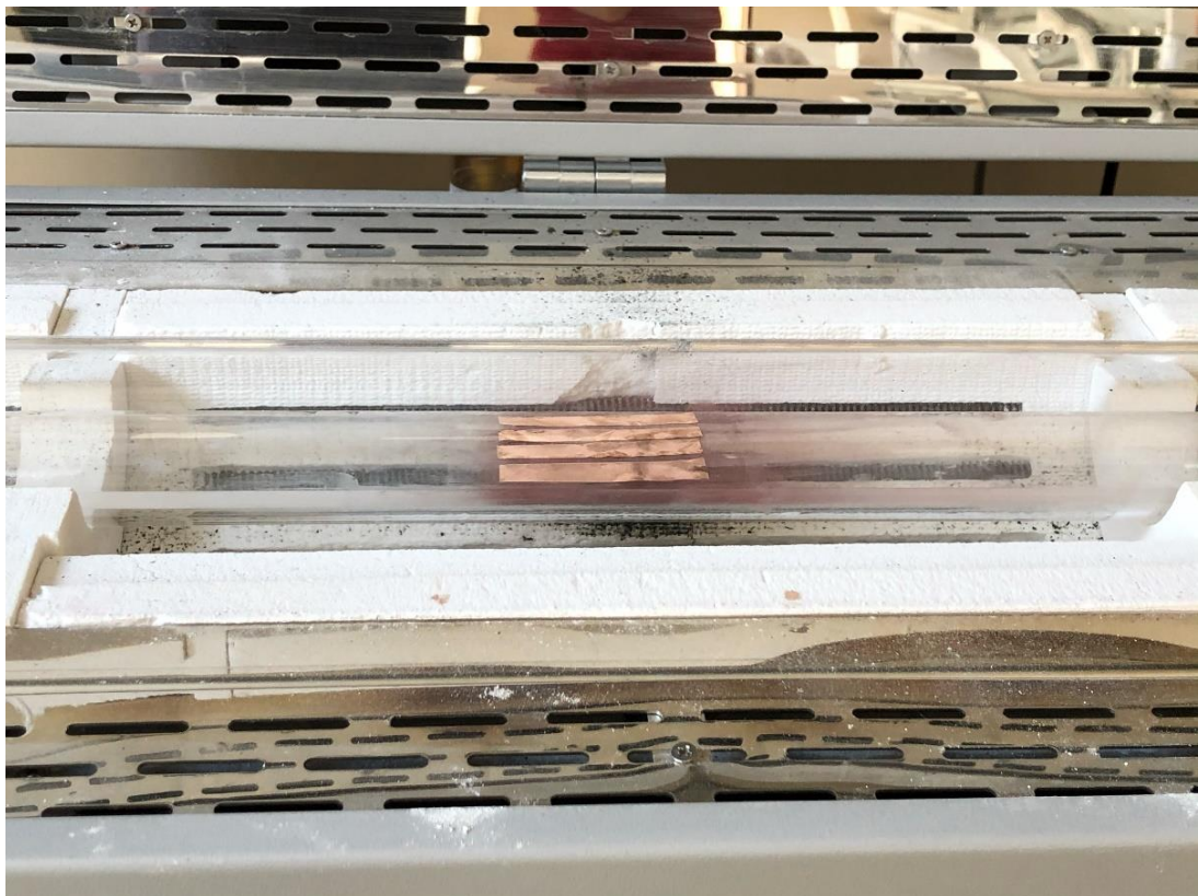
Figure 2.5: Copper substrates with graphene layer after CVD
