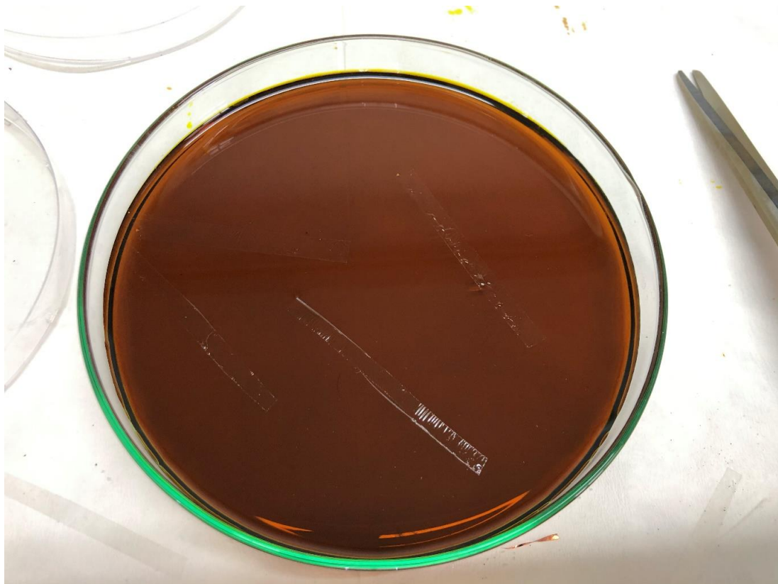
Figure 2.7: Graphene film with PMMA material
