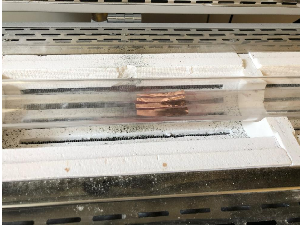
Figure 2.4: Copper substrates that are cut into proper dimensions and put into furnace
