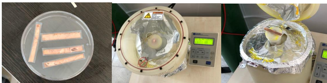
Figure 2.6: Copper substrates with graphene layer before PMMA coating (left), PMMA coating process with spin coating method (center), PMMA coated copper substrates with graphene layer (right)
