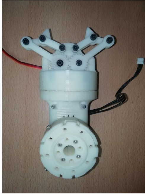
Figure 6.2 : Manufactured gripper module which is mounted to the housing part of active module
