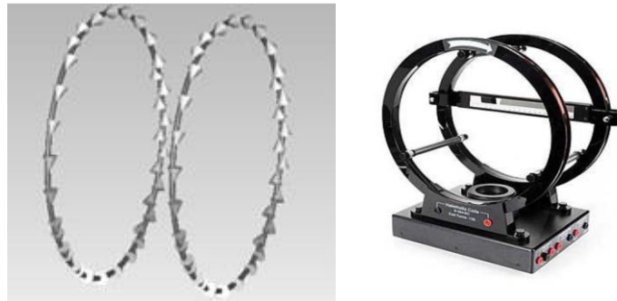
Figure 3.4: The coil design to be used in PEMF systems and the actual PASCO Helmholtz coil views.
