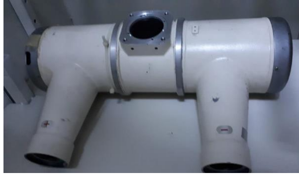
Figure 1.7: An x-ray tube sample
