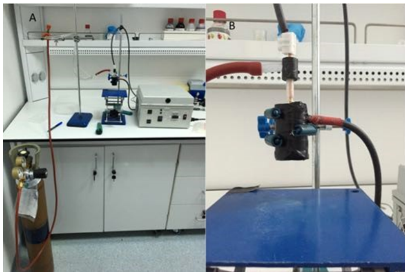
Figure 2.3: In the system for the plasma treatment, power supply, gas tube and electrode were seen (A). The supply connections which were high voltage, grounding, and gas stream (B).
