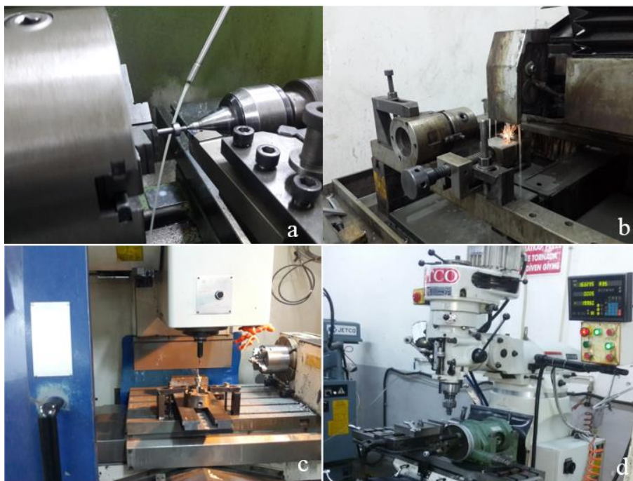
Figure 2.28: Manufacturing techniques which are used for production of transvaginal uterus amputation device. (a) Turning lathe, (b) Wire cut, (c) CNC, (d) Router.
