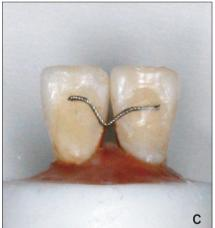
**Figure 3.** Representative acrylic blocks with embedded human incisors and wire after debonding. A, group I; B, group II; C, group III.
