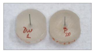
**Figure 2.** Representative acrylic blocks with embedded wire segments prepared for use in the pull-out force test.
