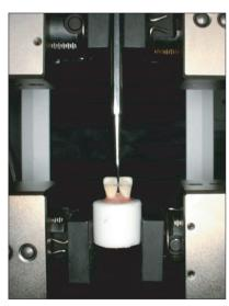
**Figure 1.** A prepared acrylic test block with embedded human incisors and bonded wire loaded into the Instron testing machine.
