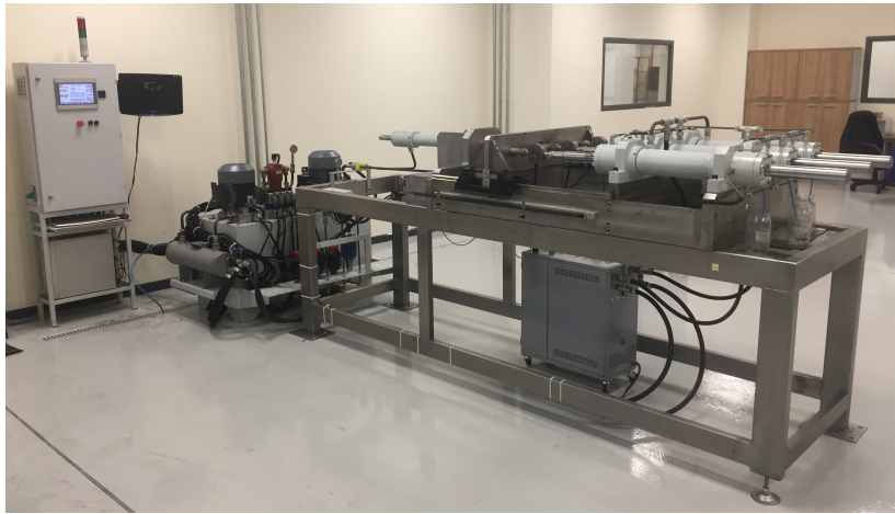
Figure 2.12: TR012013 Hydraulic rod seal test rig.
