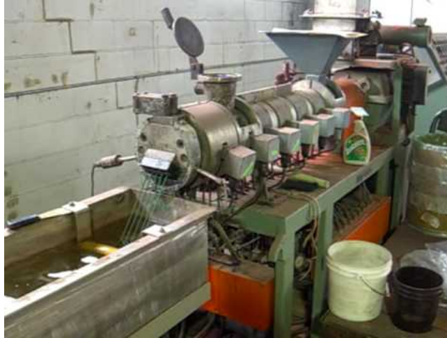
Figure 2.2: Twin screw extruder.
