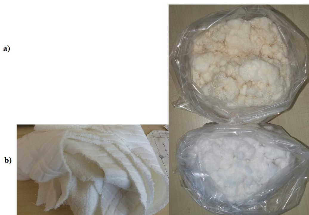
Figure 2.1: Textile wastes; a) cotton cut waste (used without shredding), b) cotton clips (unshredded (left) and shredded (right))
