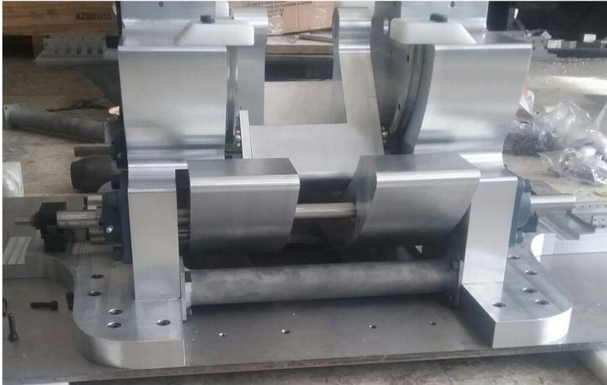
Figure 2.21: Assembly period, close up, stabilizers and circular rails are visible.
