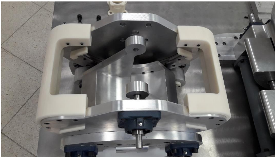
Figure 3.23: Assembling of the jaws and walls.
