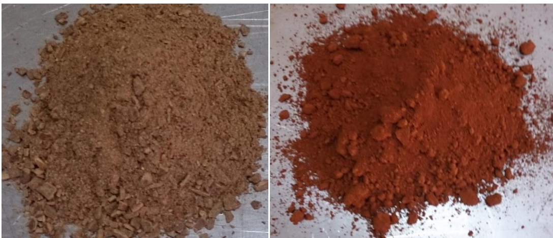
Figure 3.5: 1000 rpm and 2 min grinding for hazelnut shell and red mud.
