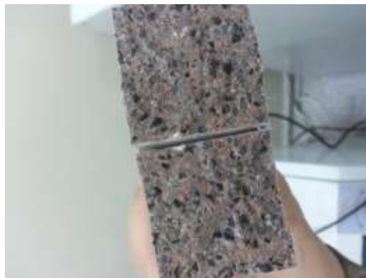
Figure 2.12 : Internal structure of specimens after failure.
