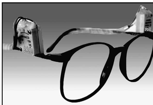
Fig 3. Cranial portion of the device. Note the placement of the inclinometers on opposite sides.
