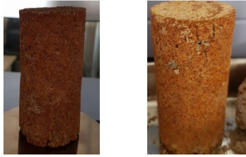
Figure 5.4 : Specimen with sulphuric acid a) before and b)after test.
