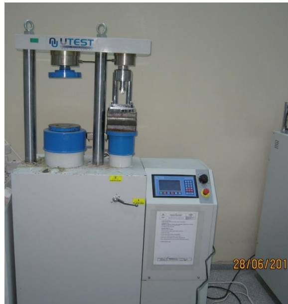
Figure 4.6 : Unconfined compressive strength test machine
