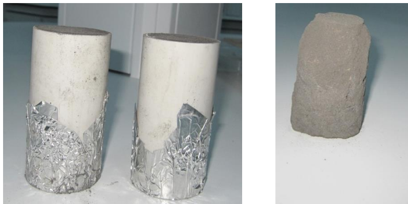
Figure 5.2 : Unmolded specimens or spread during unmolding
