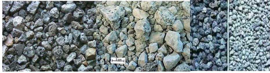
Figure 3.3 : a) Blast furnace slag b) Air-cooled blast furnace slag c) Pelletized blast furnace slag
