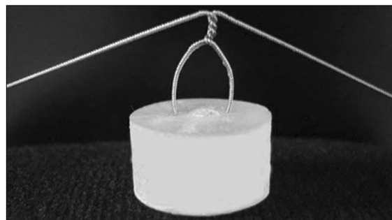
Fig 2. Prepared block for wire pull out resistance test.
