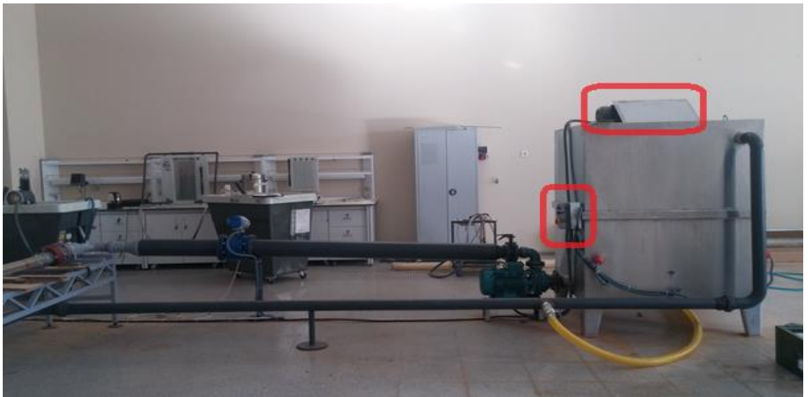
Figure 3.7 : Heater control unit and stirring motor
