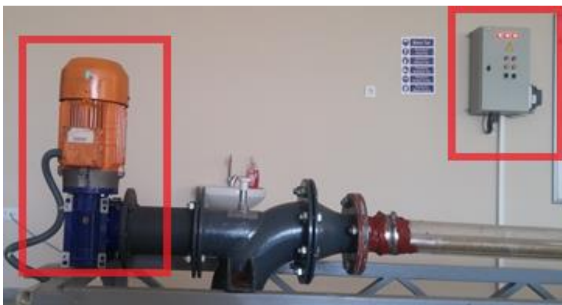
Figure 3.2 : Motor for pipe rotation and its control unit
