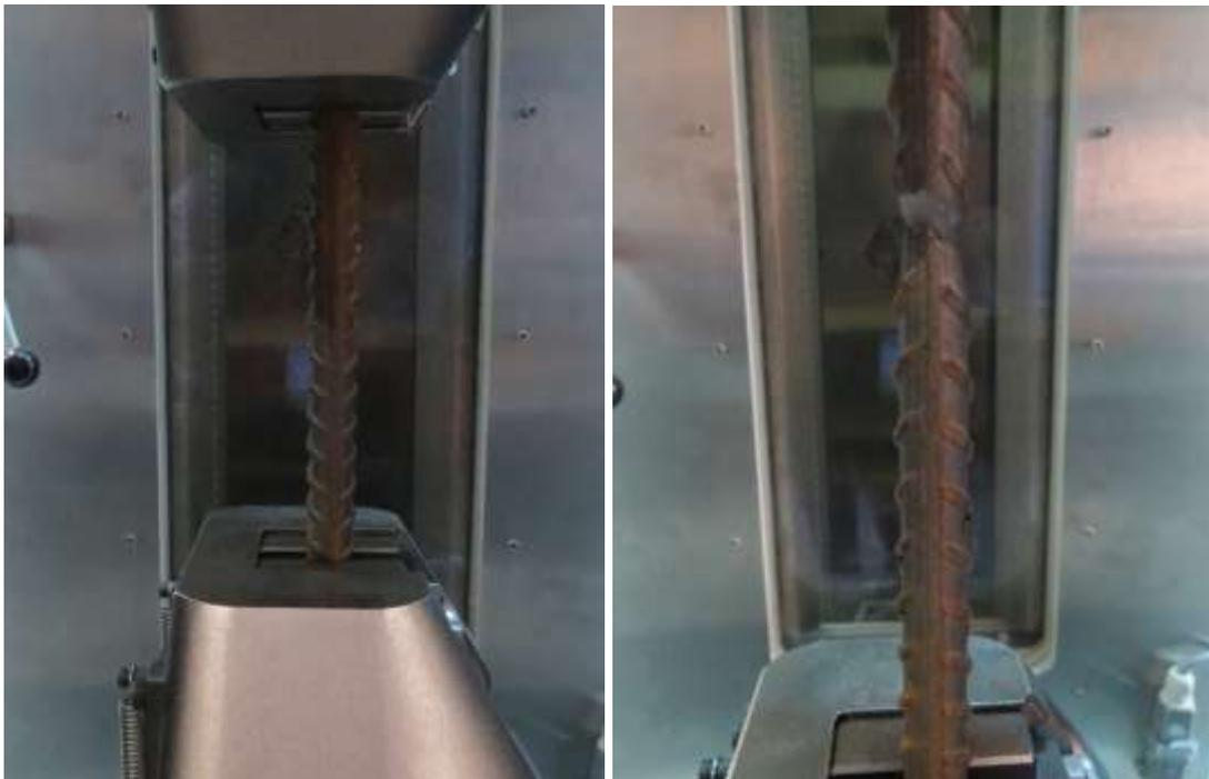
**Figure 3.8** : Tensile test of anchor bars.
