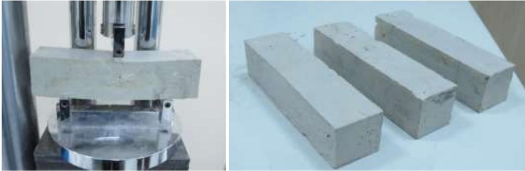
**Figure 3.10** : Flexure strength test of epoxy.
