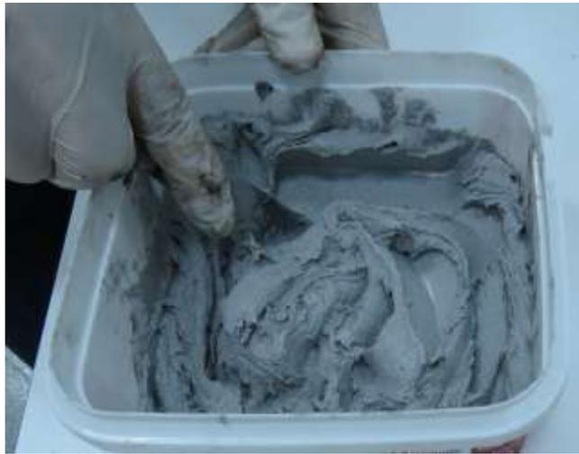
**Figure 3.4 :** Preparation of epoxy.
