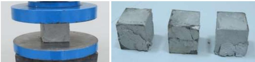
**Figure 3.11** : Compressive strength test of epoxy.
