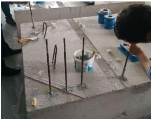
**Figure 3.5 :** Embedment of anchors.
