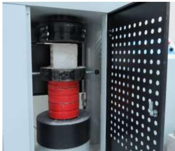
**Figure 3.7 :** Compressive strength test for concrete sample.
