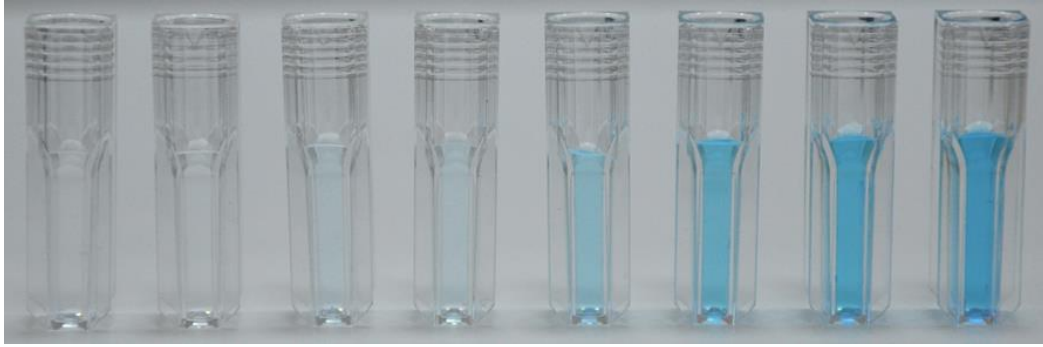
Figure 3.2: The photographic images of MB solutions from 0.1 to 10 ppm with increasing concentration and color intensity.
