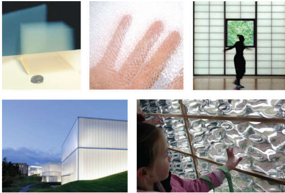
Figure 3.24 : Some examples of transparent insulation materials.
