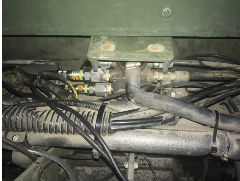
Figure 4.10 : Pressure sensors mounted on the foot brake valve of prototype vehicle.
