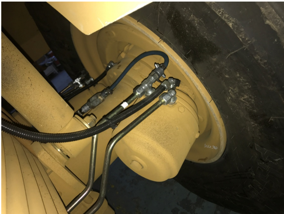
Figure 4.3 : Pressure sensor mounted on the rear axle right.
