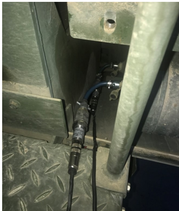
Figure 4.11 : Pressure sensors mounted on the front and rear tanks of prototype vehicle.
