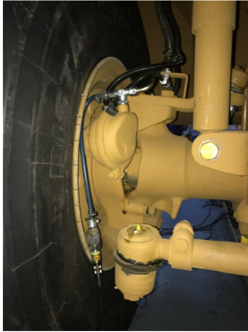
Figure 4.2 : Pressure sensor mounted on the front axle left.
