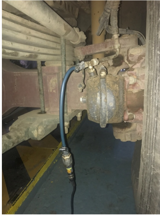
Figure 4.8 : Pressure sensor mounted on the front axle left of prototype vehicle.
