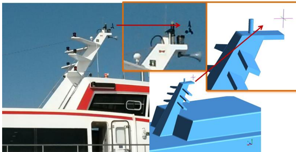
Figure 3.18 : Anemometer Sites and Details for the Real Catamaran Ship and The Model.
