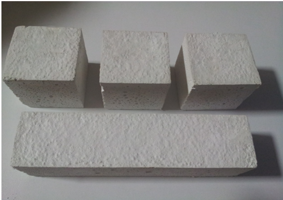
Figure 3.14 : Hardened state of the plasters.
