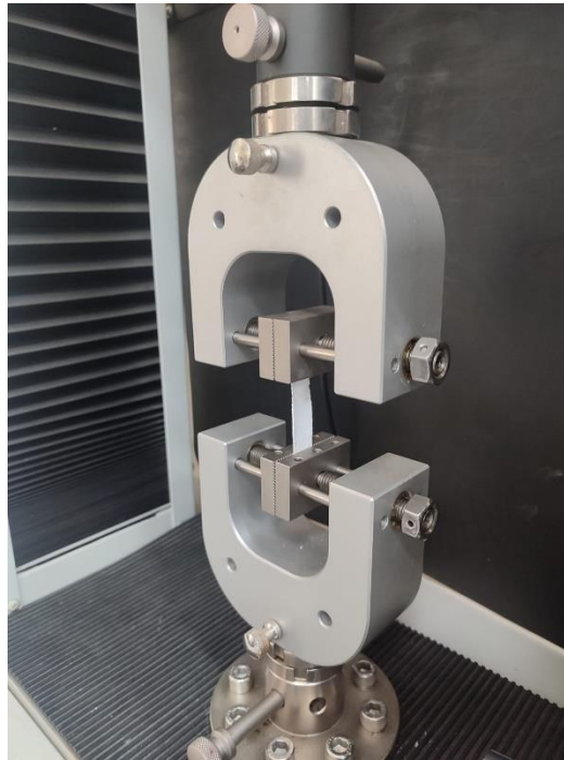
Figure 19: Setup of tensile test
