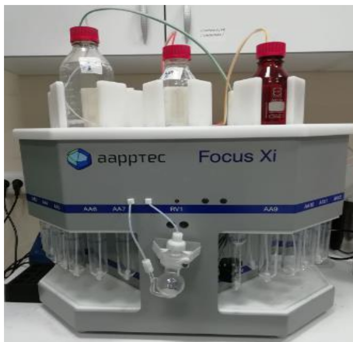
Figure 11: Peptide synthesizer (AAPPTEC LLC-Focus X).
