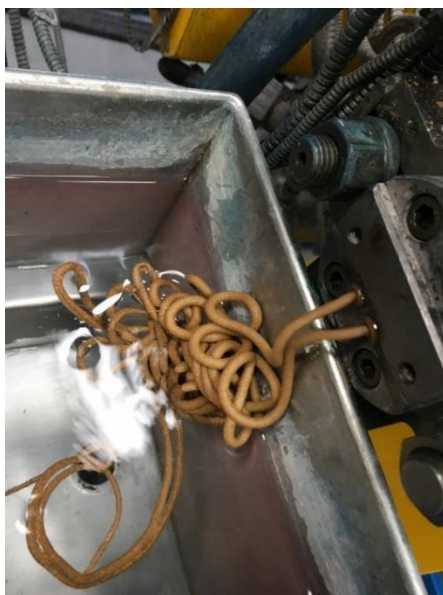
Figure 2.5: Product in spaghetti form Figure 2.6: Pellet machine
