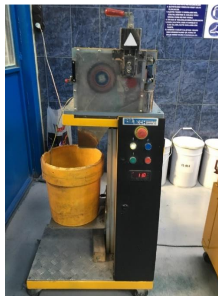
Figure 2.5: Product in spaghetti form Figure 2.6: Pellet machine
