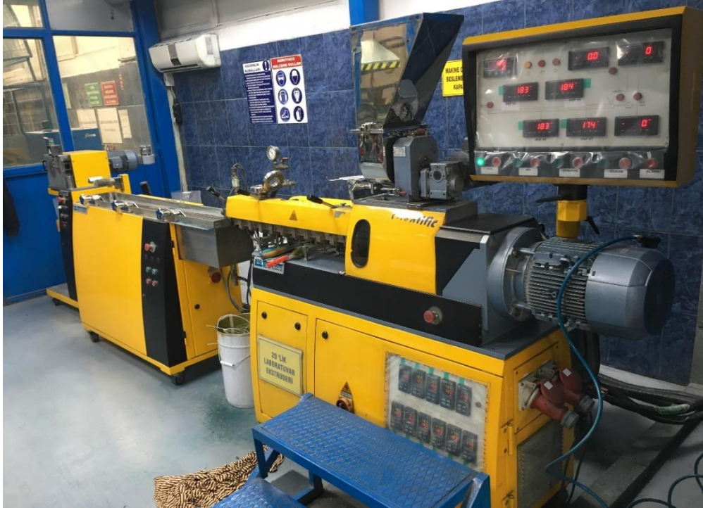
Figure 2.4: Twin screw Co-rotating Extruder
