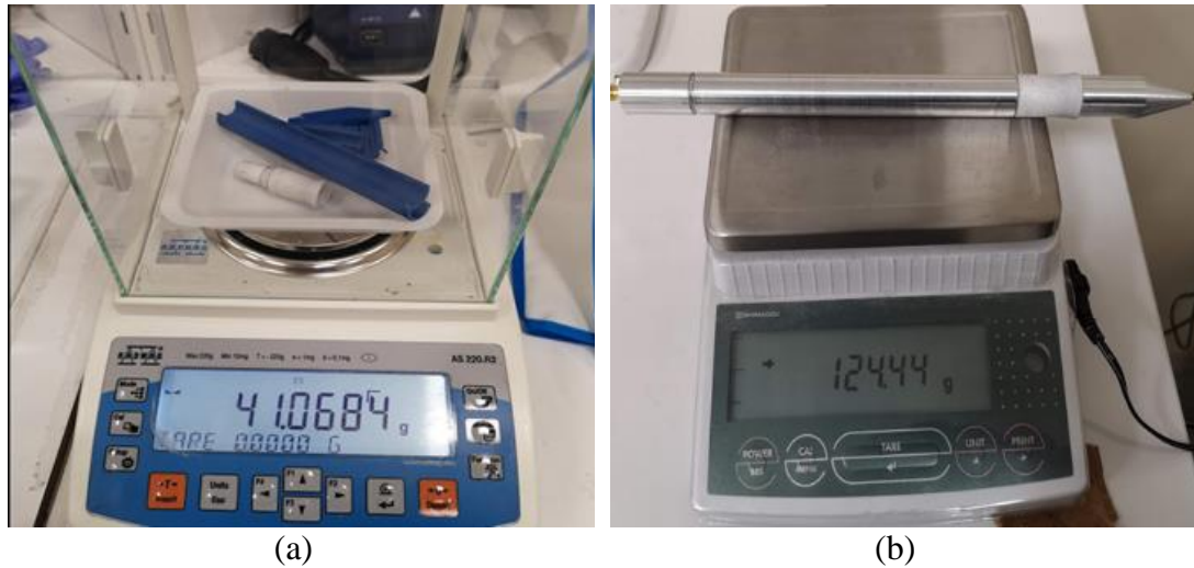
Figure 6.8: Weight measurements of microwave probes made of: (a) ABS, and (b) aluminum
