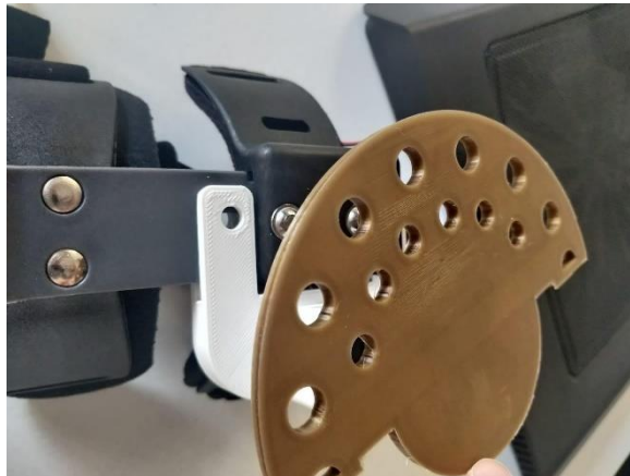
Figure 2.3: Picture of the early design of the arm (brown) placed over the motor
