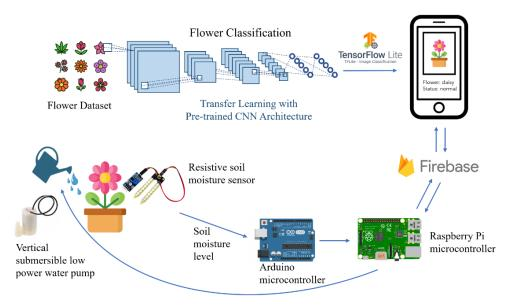
Figure 4. Schematic of the flower status tracker and self-irrigation system on smartphones.
