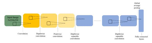
Figure 1. MobileNet V1 architecture.
