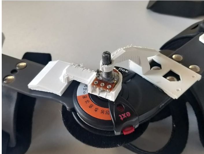
Figure 2.14: Elbow joint angle sensor holder
