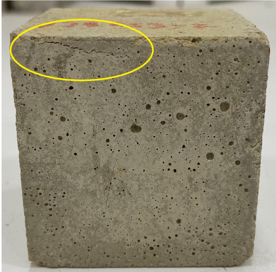
Figure 4.144: Freeze-thaw cracking on the surface of 125ES0.5 mortar
