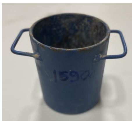
Figure 3.31: Fresh unit volume mass measurement setup
