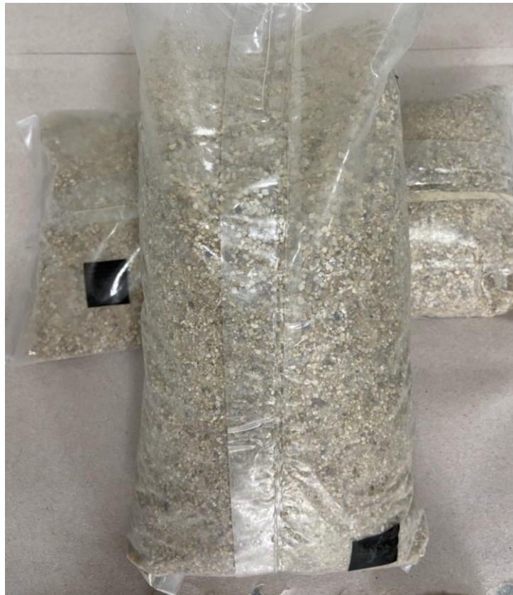
Figure 3.2: CEN standard sand used in the mixtures of mortar specimens.
