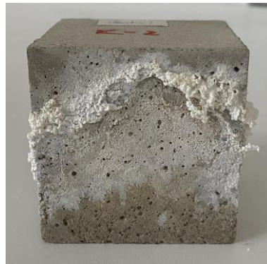
Figure 4.127: MgSO_4 bloom in reference cement mortar samples
