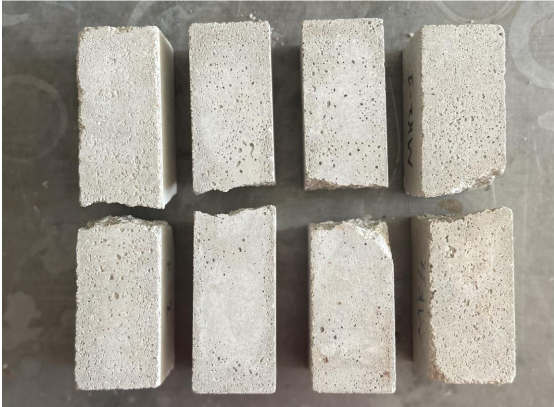
Figure 3.17: 40x40x160 mm prismatic specimens for flexural strength test.
