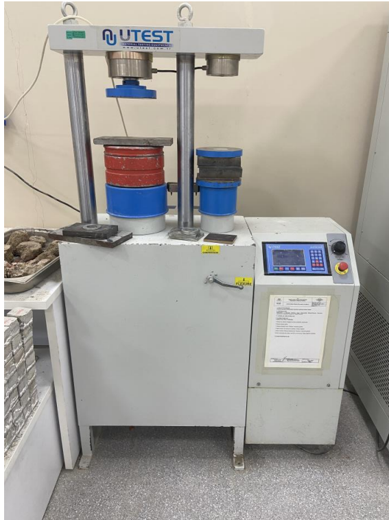
Figure 3.18: Automatic test press for compression and flexure
