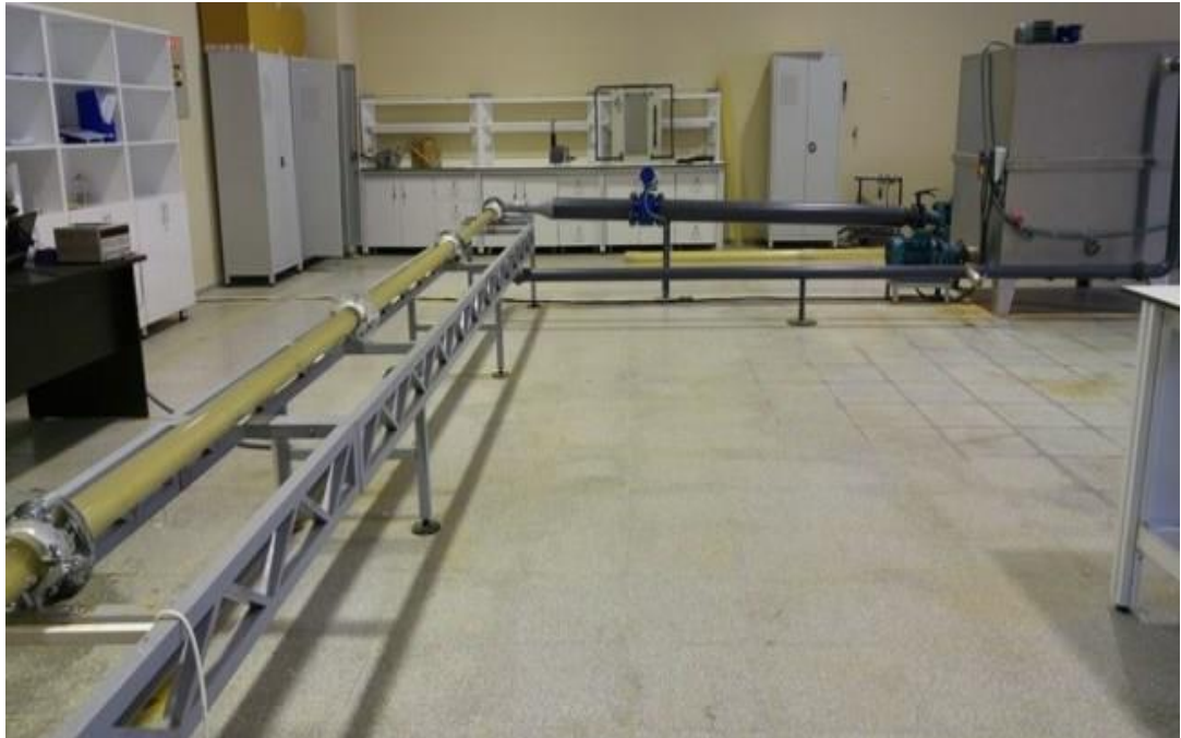
Figure 4.2 Izmir Katip Celebi University Civil Engineering Department Flow Loop, eccentric annulus.
