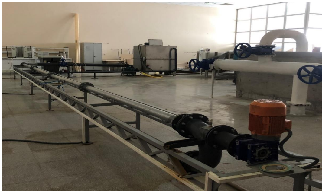
Figure 4.1 Izmir Katip Celebi University Civil Engineering Department Flow Loop, rough pipe.
