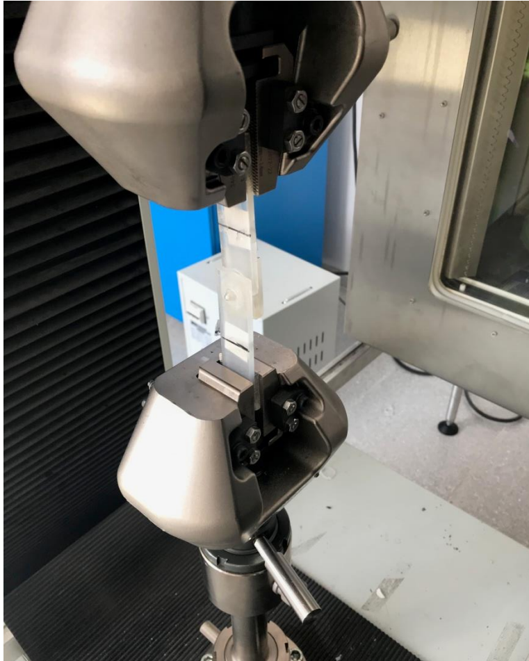
Figure 7.13 : Tensile test of a welded joint.
