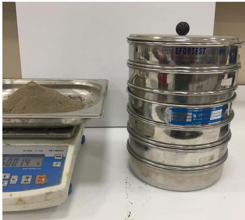
Figure 3. 5 Different size standard sieves
