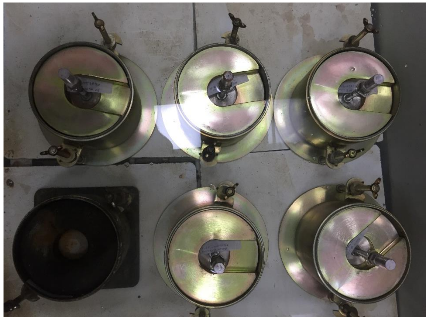
Figure 3. 16 Soaking stage of CBR test
