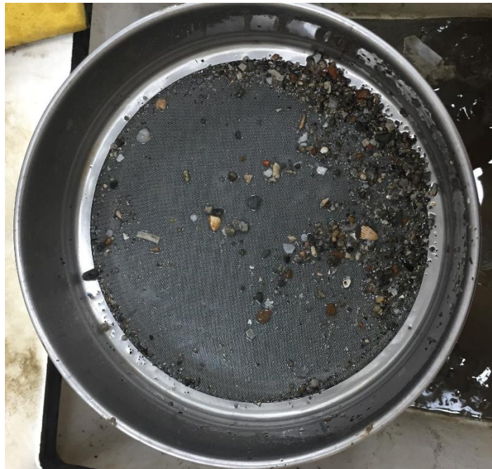
Figure 3. 6 Remained particles of F.G sample on No. 200 sieve
