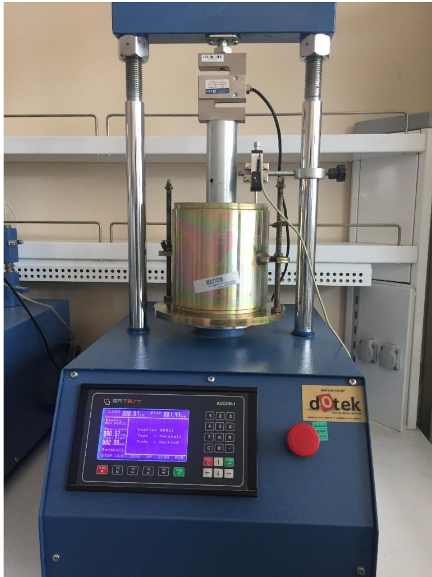
Figure 3. 17 CBR test's loading machine
