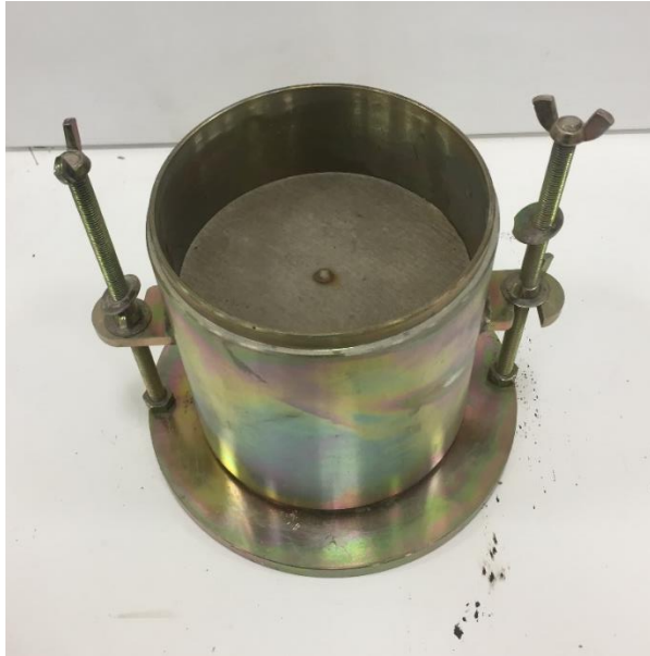
Figure 3. 15 Compacted soil sample in CBR mold
