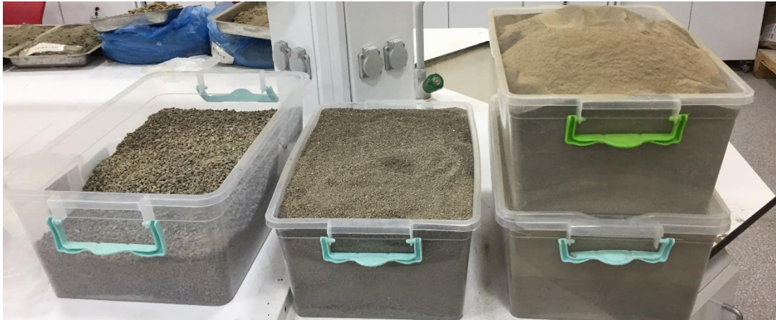
Figure 3. 2 Fine, medium, and coarse grain alluvial soil samples
