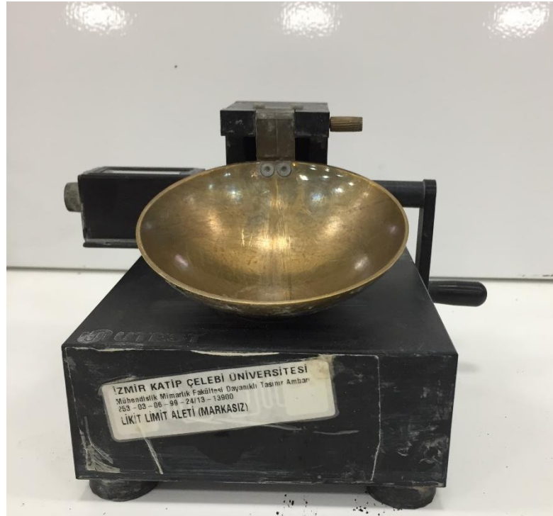
Figure 3. 11 Casagrande apparatus for liquid limit test
