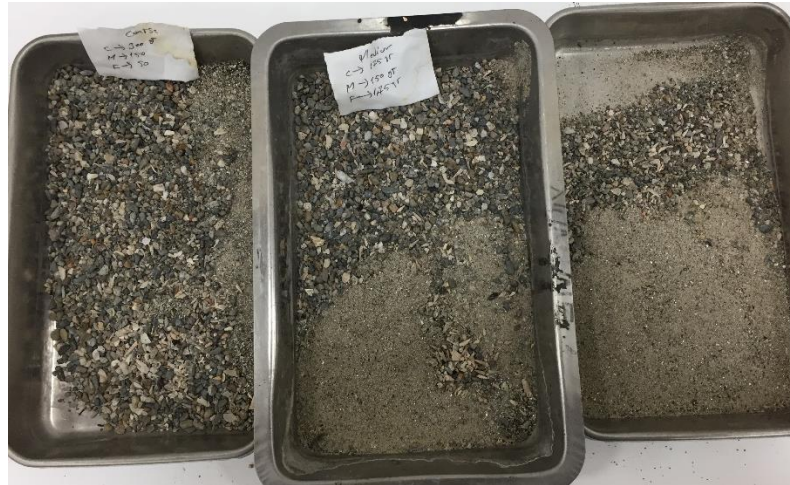
Figure 3. 7 Oven dried samples of C.G, M.G, and F.G samples after wash sieve test
