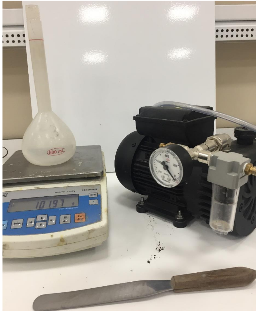
Figure 3. 8 Specific gravity test's equipment
