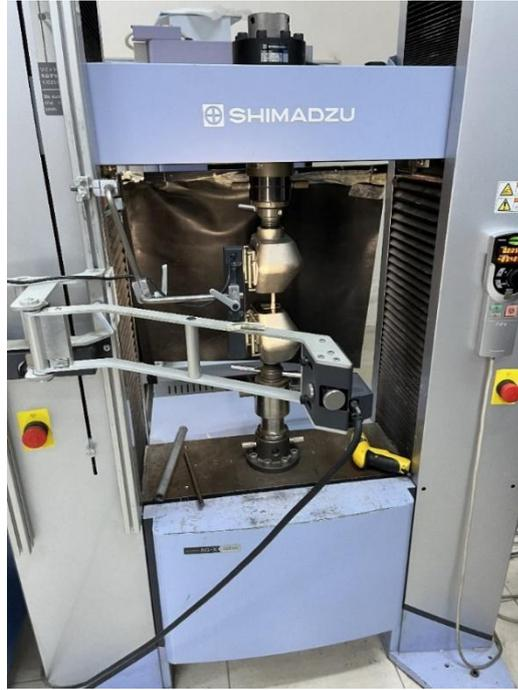
Figure 2.17: Shimadzu Tensile test machine
