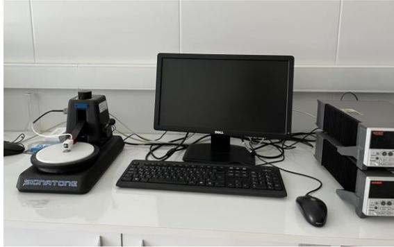
Figure 2.18: 4-point measurements apparatus
