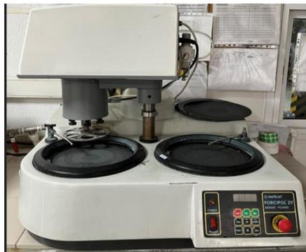
Figure 2.14: Automatic grinding & polishing machine
