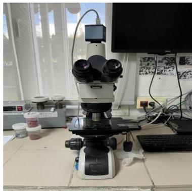
Figure 2.15: Nikon Eclipse Optical Microscope
