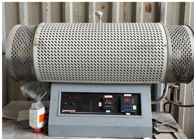
Figure 2.12: Protherm tubular furnace
