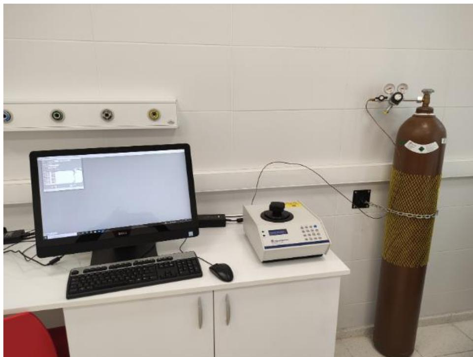
Figure 2.3: Micromeritics AccuPyc II 1340 helium pycnometer
