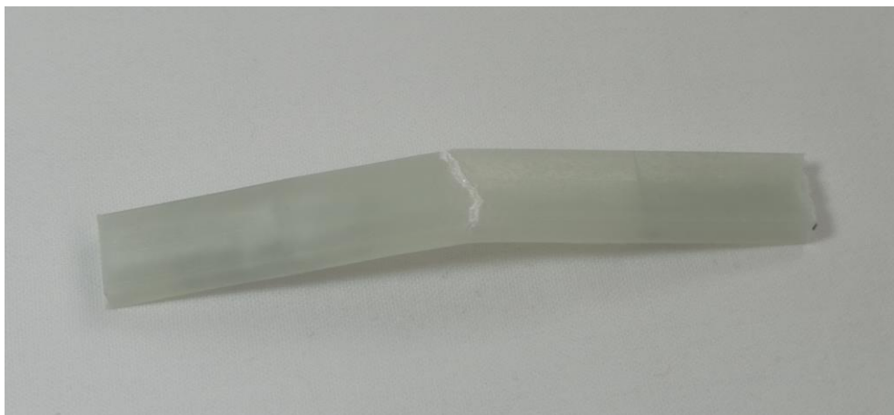
Figure 6.22: The weld line specimen made of PP GF20 after bending testing
