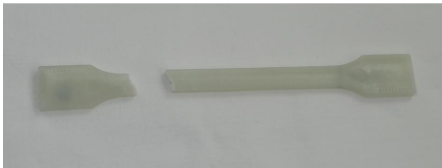
Figure 6.19: The non-weld line specimen made of PP GF20 after tensile test
