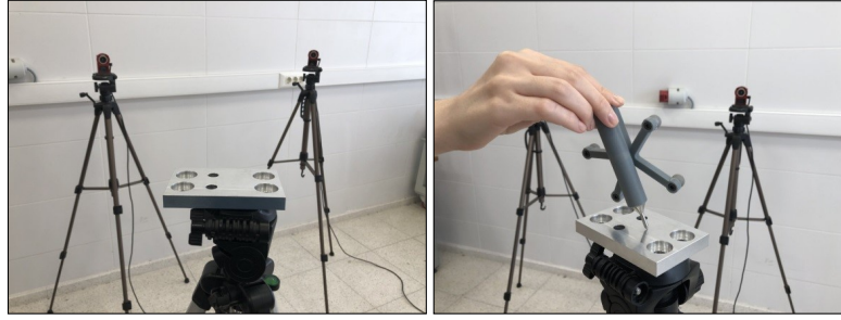
Figure 6.25. Apparatus Manufactured for Pivot Calibration and Process of Calibration.
