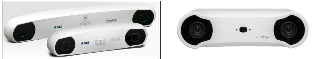
Figure 3.1. Classical Surgical Navigation Systems (NDI, Atracsys).
