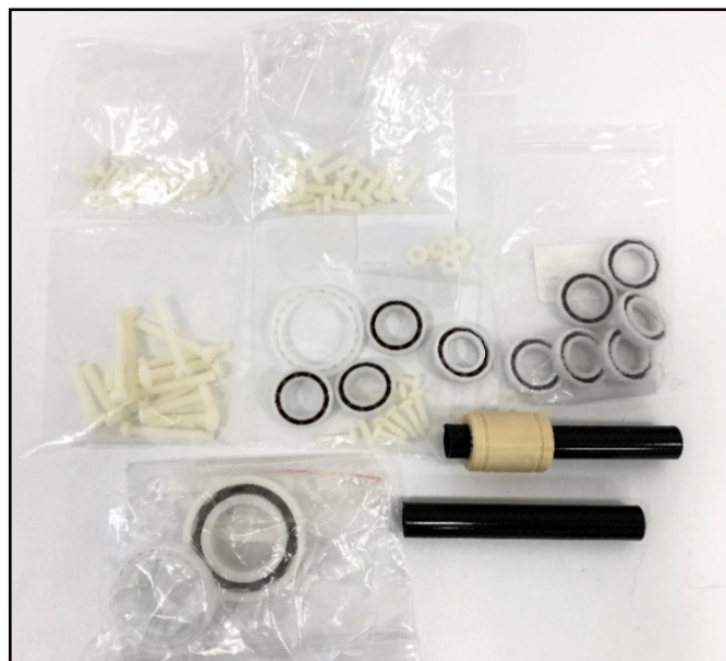
Figure 5.2: Carbon rails, glass ball bearings, teflon linear bearings and polymer fasteners
