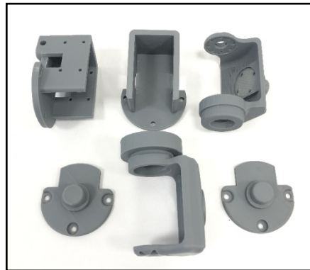
Figure 7.5: Initial prototype production trials Zortrax M200
