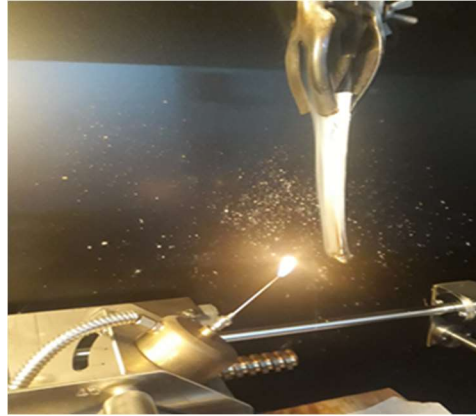
Figure 2.8 UL-94 vertical testing.
