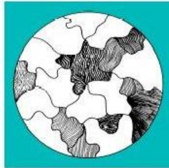
Figure 1.4: A photomicrograph of a piece of steel containing about 0.30% carbon will look something like this, showing a mixture of ferrite grains (white) and pearlite grains [1].
