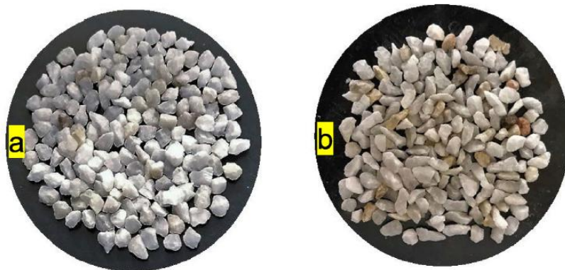
Figure 5.21 Optical microscopy images of coarse \text{CaCO}_3 particles a) well sorted, high spherical b) poor sorted, low spherical.
