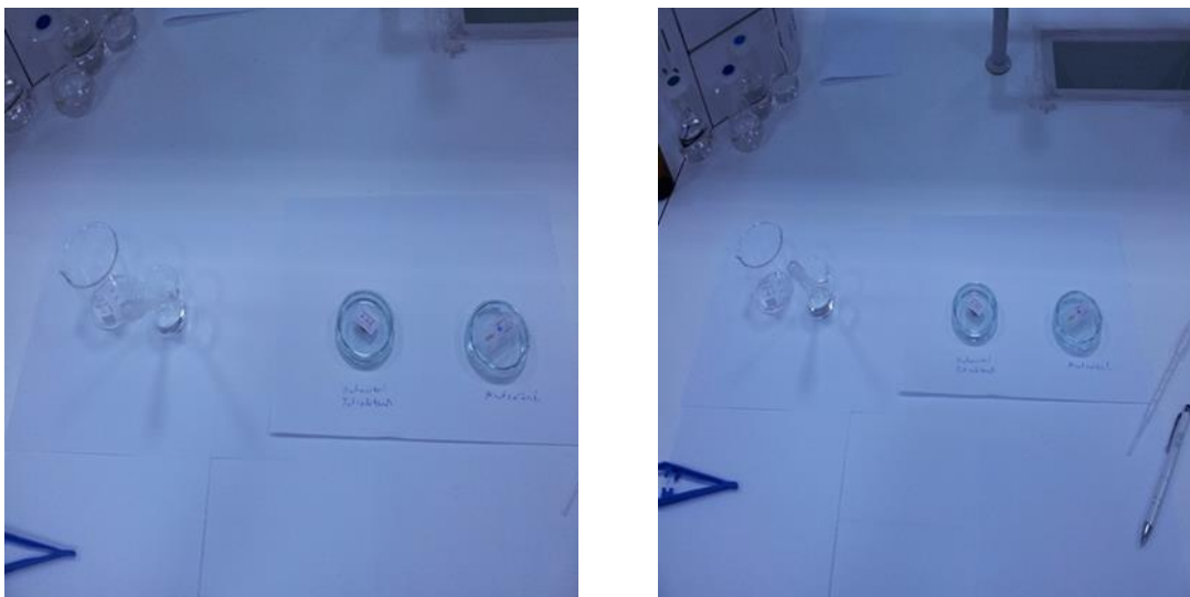
Figure 2.2: Immersion in the solvent of the counter electrode.
