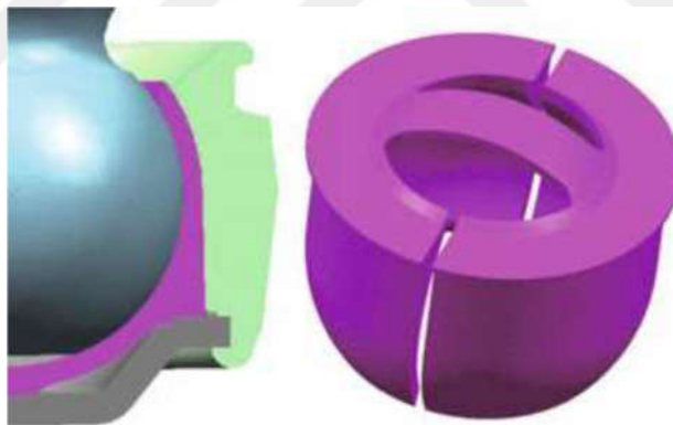
Figure 2.2: Bucket-type ball race with two slits
