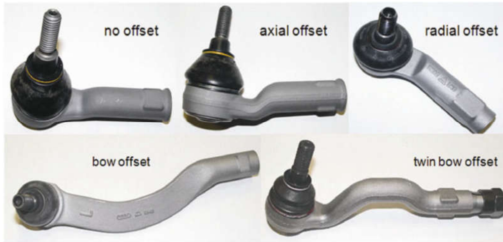
Figure 1.8: Different outer tie rod design types [1]
