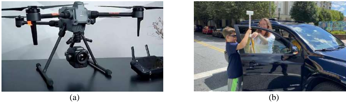
Figure 5. (a) :Image of unmanned air vehicle and thermal camera (b): Image of car-based mobile measurement system
