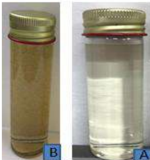
Figure 1: Color change of extract containing nanoparticles, A-extract without AgNO 3 . B- Extract with AgNPs
