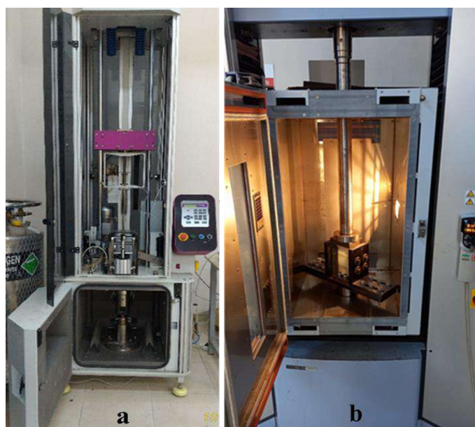
Figure 2. a) Low velocity impact device, b) CAI test setup
