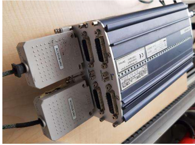
Figure 4. Multichannel datalogger unit and connections.
