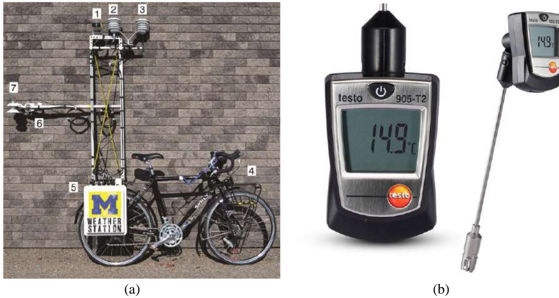
Figure 8. (a): Image of the bicycle-based mobile measurement system: 1. GPS; 2. relative humidity and air temperature; 3. air temperature; 4. sky view factor camera location (not shown); 5. Datalogger and barometric pressure; 6. Ground surface temperature; 7. Four component net radiometer. (b): Image of surface temperature meter
