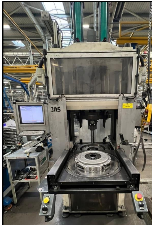
Figure 5.19: The clutch cover assembly performance test device.
