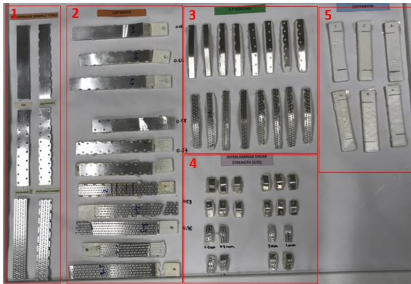
Figure 2.21: Overview of test samples 1-Aluminium sample types; 2-Lap-shear samples; 3-3P Bending samples; 4-ILSS samples; 5-Coefficient of Linear Thermal Expansion samples
