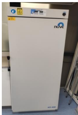
Figure 2.6: Heating oven -Nuve KD400
