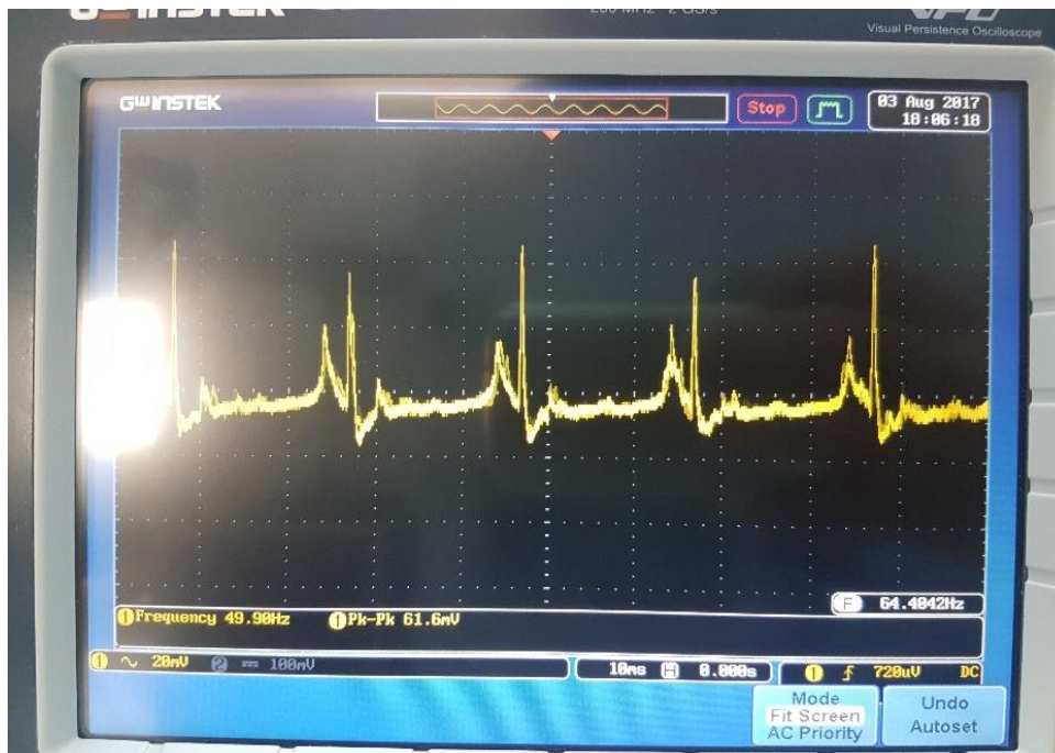
Figure 3.10 : The oscilloscope screen of an amplified and filtered ECG signal.
